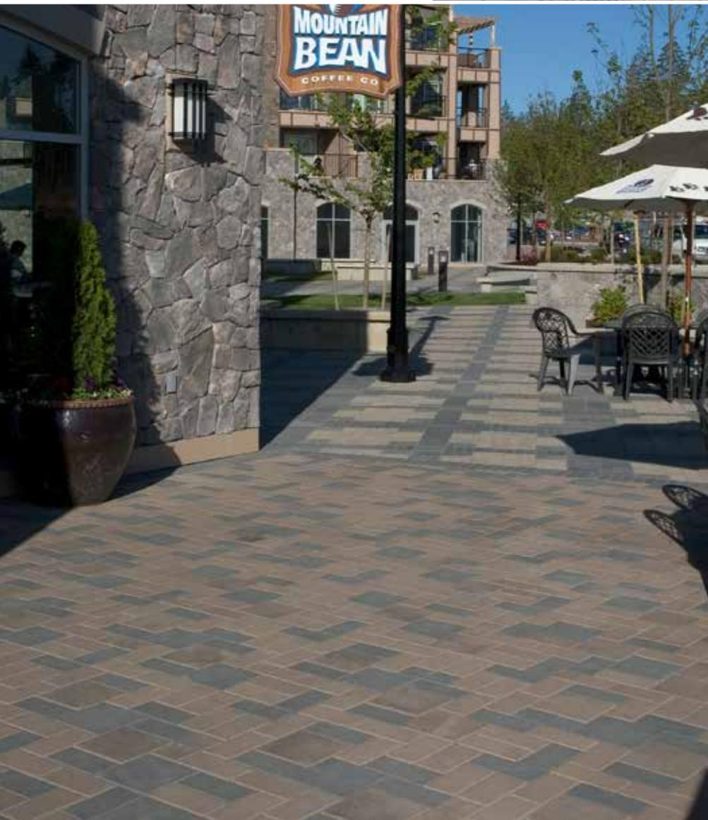
*Our pavers are made with the unique **PermaFinish** two layer process. In this process, the wearing surface of the paver is composed of uniformly graded hard, sharp granite aggregate, high cement content and a correspondingly high pigment content. This results in a dense high strength surface, more intense color stability and greater abrasion resistance than traditional paving stones. The balance of the paver is composed of high strength compressed concrete.*
